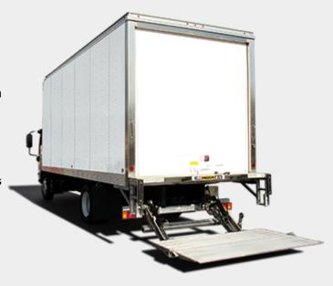
The MXT models feature a 48" x 80" wedge-type Steel, Steel/Aluminum as well as all-Aluminum platform with optional dual cart stops. Standard features include a bolt-on extension plate and steps, hydraulic locking, grease fittings at all critical rotation points and all steel components come hot-dip galvanized - **STANDARD**.
