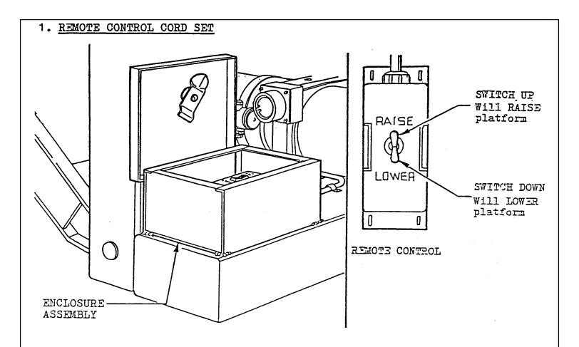
The unit is operated by a remote control cord set which is connected to a solenoid switch on the pump motor.
