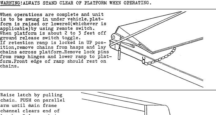
9. Raise latch by pulling chain. PUSH on parallel arm until main frame channel clears end of latch. Release chain. Grasping the platform support bar ( a 5/8" rod located between the front and the top of the platform ) PUSH the unit under the vehicle, close to (代))))))))))))))))))))))))))))))) but not against the Lock Plate and Saddle Assembly. PUSH
