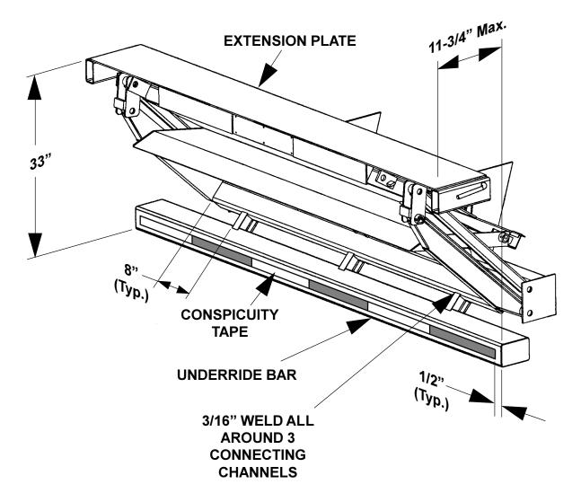
**2.** Add Conspicuity Tape to the rear face of the Underride Bar. Bring the tape to within 1/2" of each end of the Underride Bar.
