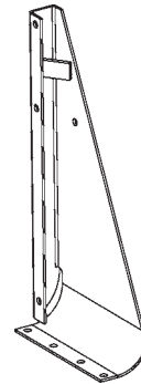
MOUNTING BRACKET WELDMENT, LH P/N 289542-01G QTY. 1
