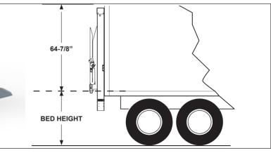
Mounting Requirement Dimensions (see installation manuals for details) NOTE: Please review appropriate liftgate installation manual for full vehicle and or body requirements to ensure proper fitment.
