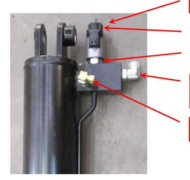
Move lock valve to new cylinder.
