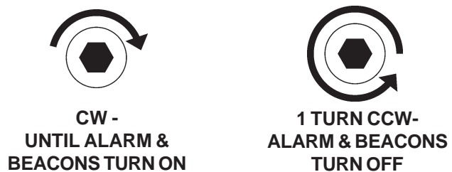
MAT SWITCH ADJUSTMENT SCREWS FIG. 15-2
