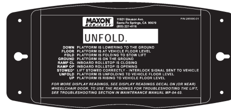
CONTROLLER READING - PLATFORM STOPPED BEFORE FOLDING FIG. 25-1
