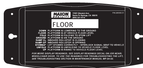
CONTROLLER READING - PLATFORM AT FLOOR LEVEL FIG. 30-3
