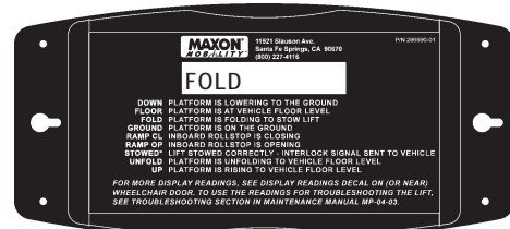
CONTROLLER READING - PLATFORM FOLDING FIG. 33-3
