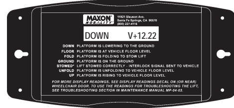
EXAMPLE CONTROLLER DIAGNOSTIC READING FIG. 83-1
