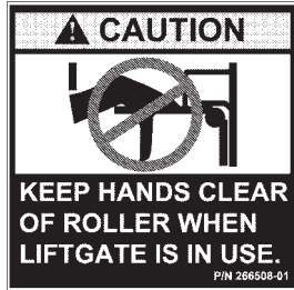
CAUTION DECAL (2 PLACES) (LABEL IS PART OF PLASTIC COVER) P/N 266508-01
