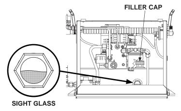
CHECKING HYDRAULIC FLUID LEVEL FIG. 18-1
