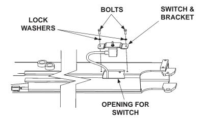
REMOVING SWITCH FROM RH RUNNER FIG. 38-1
