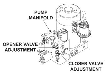
GRAVITY DOWN PUMP FIG. 22-2 THIS PAGE INTENTIONALLY LEFT BLANK.
