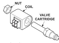
TYPICAL SOLENOID VALVE REMOVED & DISASSEMBLED FIG. 77-2
