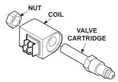
TYPICAL SOLENOID VALVE REMOVED & DISASSEMBLED FIG. 81-1
