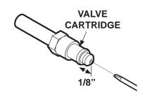
CHECKING VALVE CARTRIDGE FIG. 69-3
