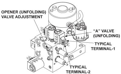
TYPICAL VALVES & ELECTRICAL CONNECTIONS
