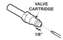
CHECKING VALVE CARTRIDGE FIG. 77-3
