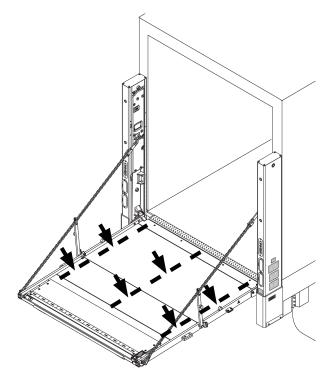
ARROWS INDICATE WHERE TO CHECK IF PLATFORM & FLIPOVER ARE FLUSH FIG. 26-1
