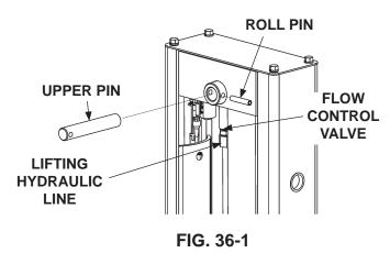
14. Lower cylinder slowly a few inches to gain access to hydraulic line connector. Plug the lifting line to prevent cylinder from compressing.
