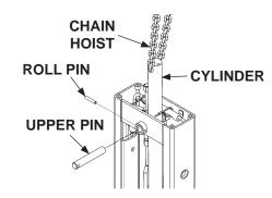
REMOVING CYLINDER FIG. 30-2
