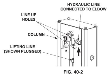
23. Remove plug from lifting line (FIG. 40-2). Then, raise the cylinder to line up the holes on cylinder and column.
