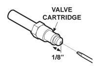
CHECKING VALVE CARTRIDGE FIG.67-3
