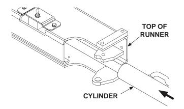
**INSERTING CYLINDER IN RUNNER** FIG. 39-1
