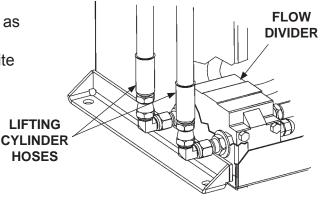
HOSE CONNECTIONS ON FLOW DIVIDER FIG. 63-1
