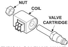
TYPICAL SOLENOID VALVE REMOVED & DISASSEMBLED FIG. 74-2
