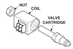
TYPICAL SOLENOID VALVE REMOVED & DISASSEMBLED FIG. 69-2
