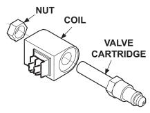
TYPICAL SOLENOID VALVE REMOVED & DISASSEMBLED FIG. 58-2
