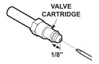
CHECKING VALVE CARTRIDGE FIG. 58-3
