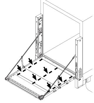
ARROWS INDICATE WHERE TO CHECK IF PLATFORM & FLIPOVER ARE FLUSH FIG. 24-1
