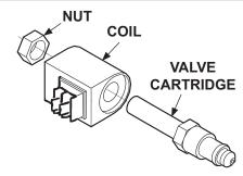
TYPICAL SOLENOID VALVE REMOVED & DISASSEMBLED FIG. 54-1
