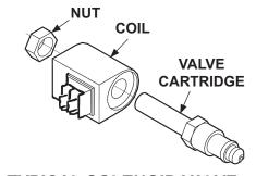
TYPICAL SOLENOID VALVE REMOVED & DISASSEMBLED FIG. 60-2
