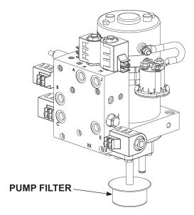
TYPICAL PUMP/MOTOR REMOVED TO CHECK FILTER FIG. 55-1
