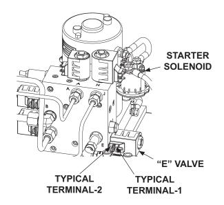
STARTER SOLENOID, VALVES & ELECTRICAL CONNECTIONS FIG. 66-1
