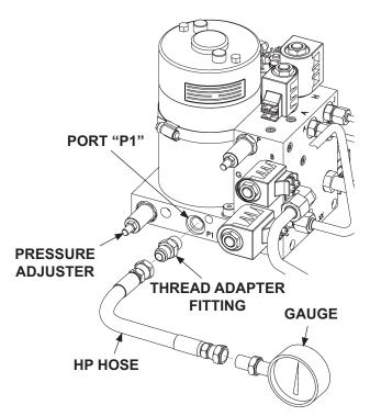
GAUGE CONNECTION AND PRESSURE ADJUSTER ON PORT PLATE FIG. 61-1
