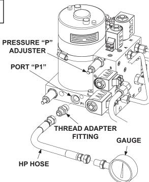
GAUGE CONNECTION AND PRESSURE ADJUSTER ON PORT PLATE FIG. 62-1
