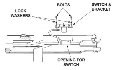
REMOVING SWITCH FROM RH RUNNER FIG. 38-1
