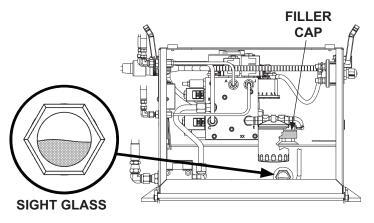
CHECKING HYDRAULIC FLUID LEVEL FIG. 16-1
