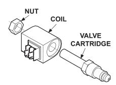
TYPICAL SOLENOID VALVE REMOVED & DISASSEMBLED FIG. 67-2
