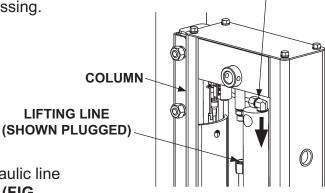
15. Disconnect power down hydraulic line from elbow on top of cylinder (FIG. 36-2). Then, cap the elbow.
