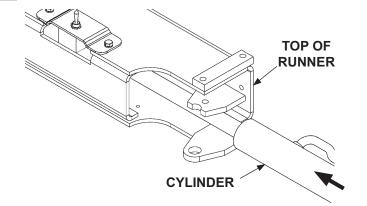
INSERTING CYLINDER IN RUNNER FIG. 39-1
