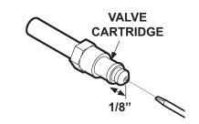
CHECKING VALVE CARTRIDGE FIG. 65-2
