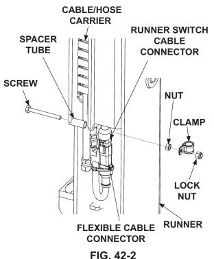
31. To reinstall opening/closing cylinder, do the opening/closing cylinder replacement steps in the OPENING/CLOSING CYLINDER REPLACEMENT procedure in this manual.
