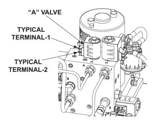
TYPICAL PUMP/MOTOR VALVES & ELECTRICAL CONNECTIONS FIG. 59-1
