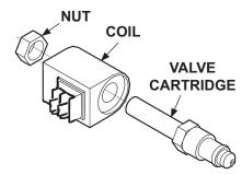
TYPICAL SOLENOID VALVE REMOVED & DISASSEMBLED FIG. 65-1
