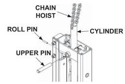
REMOVING CYLINDER FIG. 30-2
