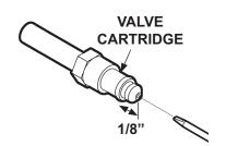
CHECKING VALVE CARTRIDGE FIG. 54-2
