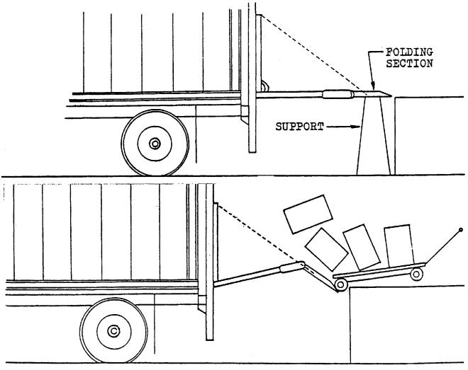
IF A SUPPORT IS NOT USED UNDER THE FOLDING PLATFORM SECTION "THIS WILL OCCUR"
