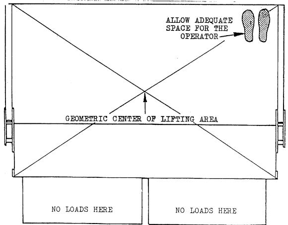
WARNING! UNDER NO CIRCUMSTANCES IS ANY LOAD TO BE CARRIED ON ANY RAMP WHICH MAY BE INSTALLED TO YOURS PLATFORM.
