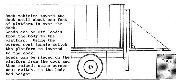
NEVER TRY TO TRANSFER LOADS FROM THE DOCK TO THE FOLDING SECTION OF THE PLATFORM OR FROM THE FOLDING SECTION OF THE PLATFORM TO THE DOCK WITHOUT FIRST PLACING A SUPPORT UNDER THE FOLDING SECTION OF THE PLATFORM, AS SHOWN BELOW. THIS ALSO APPLIES WHEN TRANSFERRING A LOAD FROM ONE VEHICLE TO ANOTHER.
