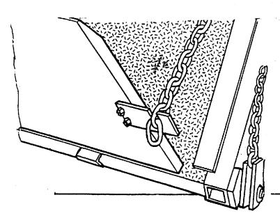
If loading is to take place with the platform lowered the retention ramp is unfolded so that it will act as a loading ramp. If loading is taking place at bed height, the ramp is placed in the bracket on the side of the ramp. The opposite end of the ramp will be secured in the same manner. The loading requirements are the same whether the platform is loaded from the ground, from bed height or from a dock.
