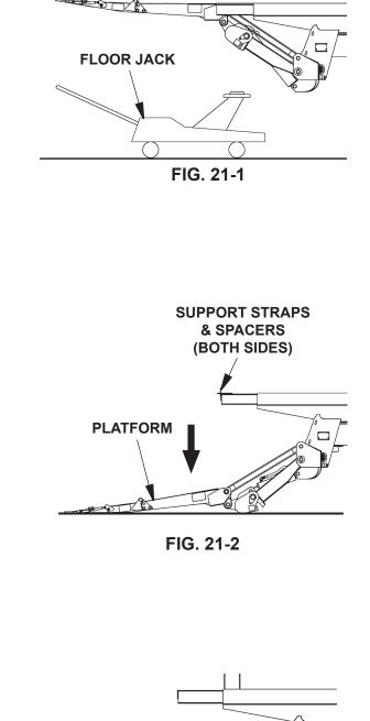
2. Lower the platform to the ground. Remove both support straps and both spacers from extension plate (FIG. 21-2).
