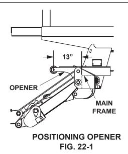
5. Fold the platform against opener (FIG. 22-2A). Make sure opener is entered on protective plate as shown in FIG. 22-2B. Reposition the opener if necessary. Clamp opener to main frame.
