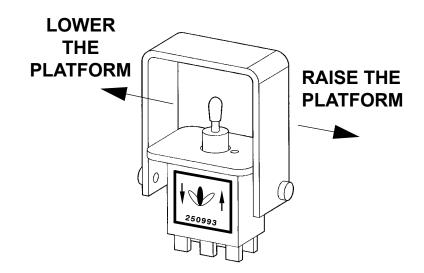
**5.** To fold the liftgate for transport, reverse steps 1 through 3. **NOTE:** It will not be necessary to hold the control handle in an "up" position to raise the liftgate. The spring loaded Hook should snap and lock onto the platform for proper storage.
