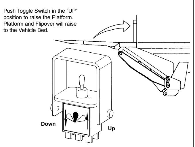
When the Platform reaches the bed height, release the "UP" switch. DO NOT CONTINUE TO HOLD THE SWITCH IN ITS RAISED POSITION. THIS WILL BURN OUT THE PUMP MOTOR.
