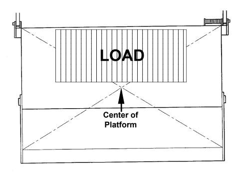
Before lifting load, check that there are no people close to the Liftgate, especially children. Accidents can occur when unstable loads topple off the lifting area and people are in close proximity to the lifting operation.
