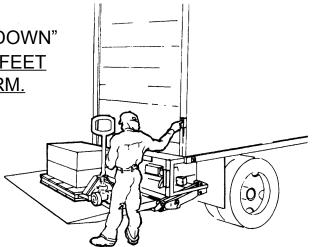
**2.** When lift touches the ground, release the toggle switch.
