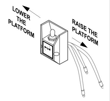
**6.** To fold the liftgate for transport, reverse steps 1 through 4. **NOTE:** It will not be necessary to hold the control handle in an "up" position to raise the liftgate. The spring loaded Hook should snap and lock onto the platform for proper storage.
