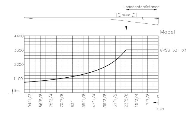
The maximum loading capacity specified in the loading diagram must not be exceeded. The platform may not be used as a bridge plate.
