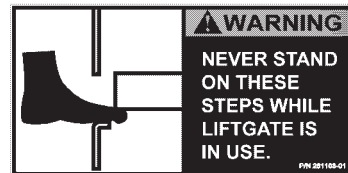
CAUTION DECAL, DUAL STEP (APPLIED AT FACTORY) P/N 281103-01 QTY. 1
