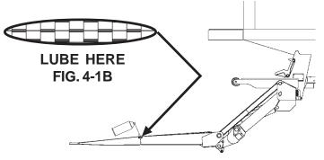
FLIPOVER UNFOLDED (GPT SHOWN) FIG. 4-1A
