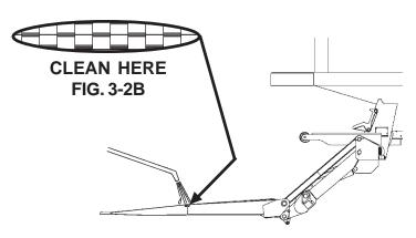
6. Dry up water from around the hinge (FIGS. 3-2A & 3-2B).
