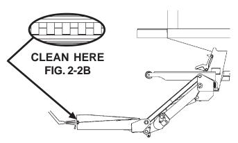
PLATFORM UNFOLDED (GPT SHOWN) FIG. 2-2A
