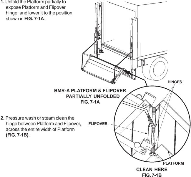
3. Dry up water from the hinge (FIG. 7-1B).
