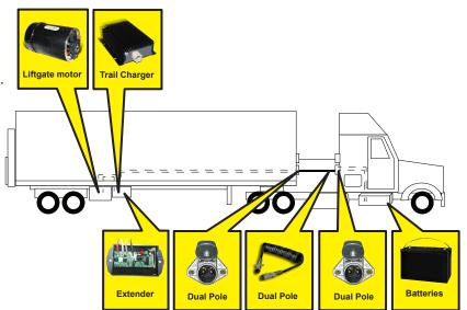
Trailer – Dry Freight Retrofit (existing single and/or dual pole wiring)
