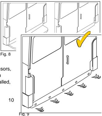
because the lifting gear interferes with the sensors (see Fig. 9).
