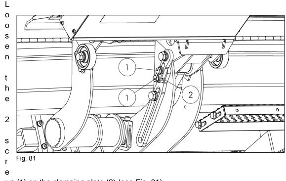
ws (1) on the clamping plate (2) (see Fig. 81).
