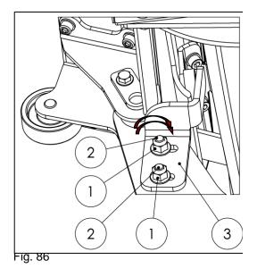
Adjust the support arm (1) so that it can be pulled as close to the vehicle as desired when the platform is closed. The adjustment is made outside at the Bowden cable (2) and, if applicable, also at the screw on the lever (3). While making the adjustment, release the Bowden cable (2) and open the platform (see Fig. 87).
