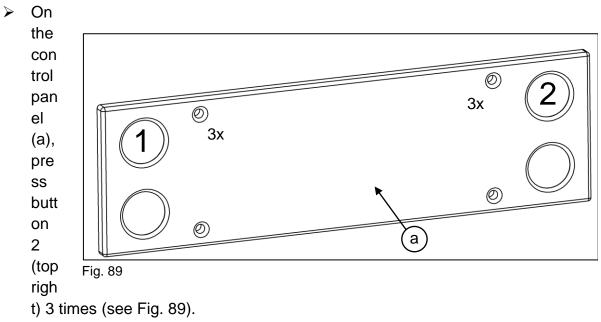
**IMPORTANT:** Each of the programming sequences with button 1 and then button 2 must be completed within a period of 2 seconds.
