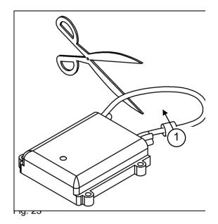
Strip the end of the control unit cable section with a red marking for connecting the handheld control (see Fig. 24).
