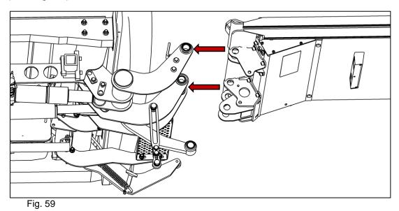
Insert the two pins (a, b) through the top attachment points of the platform and the attachment points of the swing-arm assembly.
