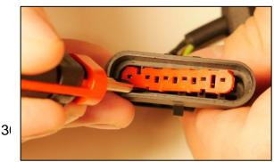
For the pin housing, release the latches on the contact pins and pull the wires out of the back of the housing (Fig. 45 and Fig. 46).
