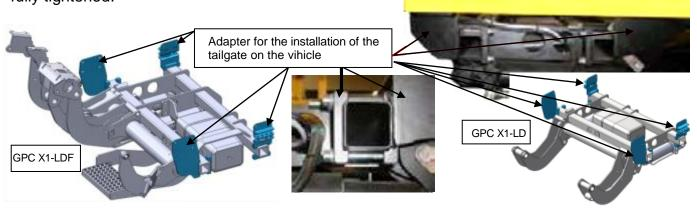
The mounting adapters on the lifting gears main frame can be adjusted sideward to assure the correct positioning of the tailgate.
