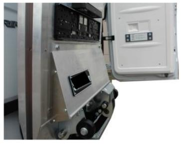
The control panel can be mounted on the inside of the right door.
