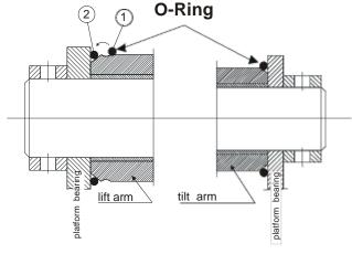
All bushing connections are sealed with an O-Ring sealing. For mounting the platform locate the O-Rings on both sides of the lift and tilt arm in Pos. 1.
