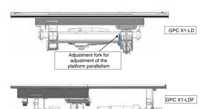
Adjustment fork for adjustment of the Platform parallelism
