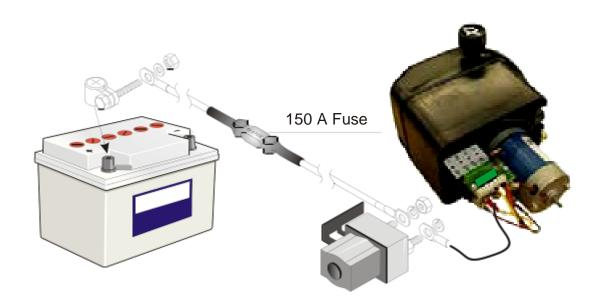
The plus cable and the ground cable are mounted on to the power pack from the factury. The shall be routed to the right poles on the battery, hereby comply to the construction guidelines of the vehicle manufacturer. The ground cable is blue and the Plus cable is red. Take care that no chafe marks are made, and that the cables are not close to heat carrying objects.
