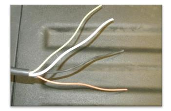
STEP 8 Cut about 8 inches off the jacketed portion off of the 4 wires.
