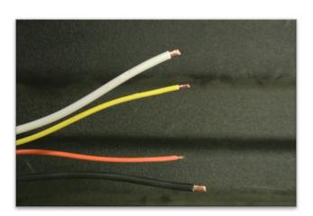
**STEP 10**Strip 3/8 of an inch of insulation off all 4 wires.
