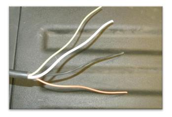
**STEP 8**Cut about 8 inches off the jacketed portion off of the 4 wires.
