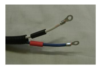
STEP 5 Crimp the supplied 10GA #10 eyelets onto both the blue and white wires.
