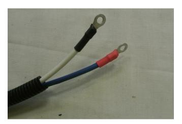
STEP 6 Solder the crimped connection then position the heat shrink over the crimps and apply heat to the 2 terminals.
