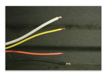
**STEP 15**Strip 3/8 of an inch of insulation off all 4 wires.
