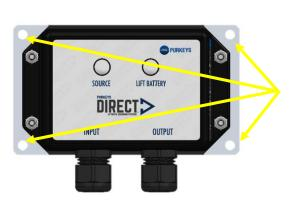
NOTE: If the L bracket is not used then the Direct<sup>™</sup> controller should be mounted to the front of the trailer via the mounting holes on the plate.
