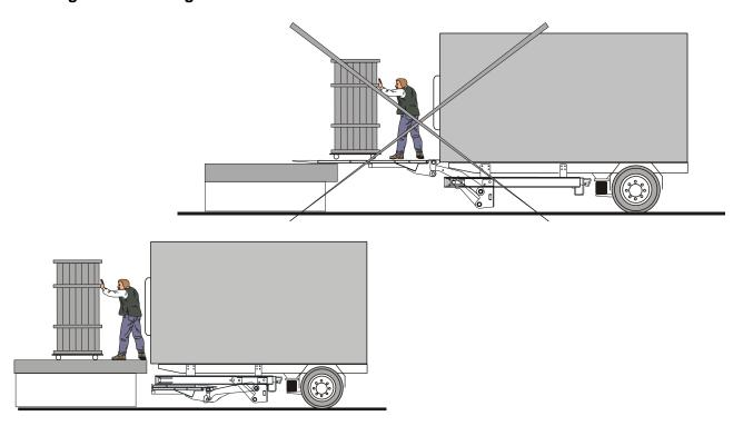
Only when the Slidelift is retracted under the vehicle.
