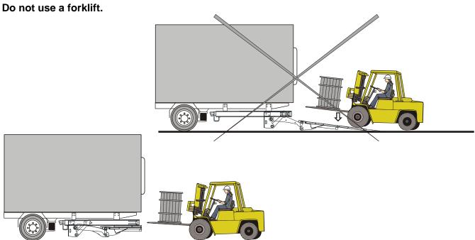
Only when the Slidelift is retracted under the vehicle.
