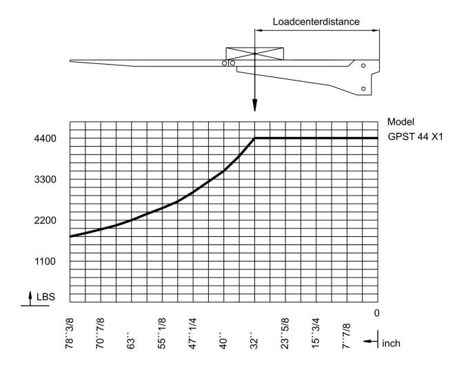
The maximum loading capacity specified in the loading diagram must not be exceeded. The platform may not be used as a bridge plate.
