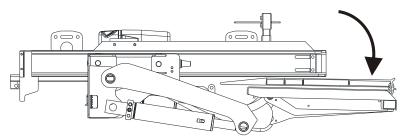
No contact between sliding frame and platform
