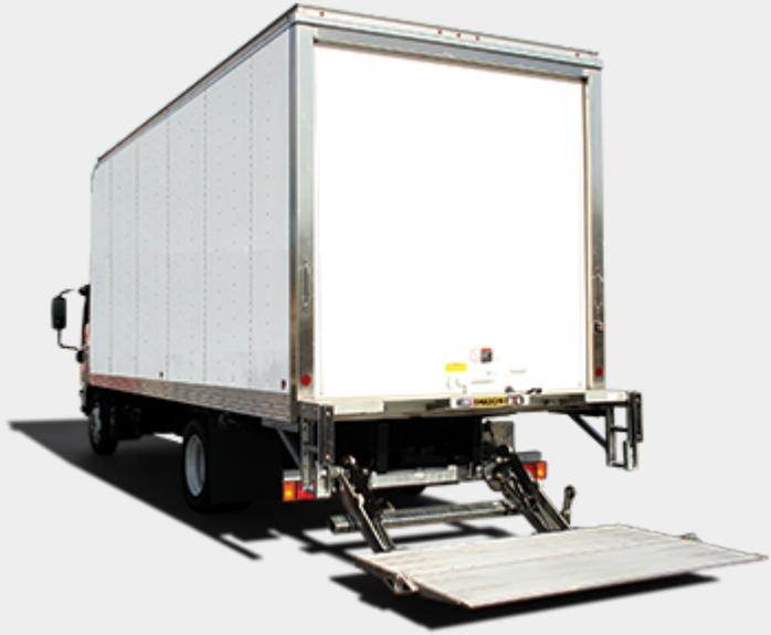
The MXT models feature a 48” x 80” wedge-type Steel, Steel/Aluminum as well as all-Aluminum platform with optional dual cart stops. Standard features include a bolt-on extension plate and steps, hydraulic locking, grease fittings at all critical rotation points and all steel components come hot-dip galvanized - **STANDARD**.
