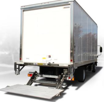
Both MXT-25 and MXT-33 models feature a 48" x 80" wedge-type Steel, Steel/Aluminum as well as all-Aluminum platform with optional dual cart stops. Standard features include a bolt-on extension plate and steps, hydraulic locking, grease fittings at all critical rotation points and all steel components come hot-dip galvanized - STANDARD.
