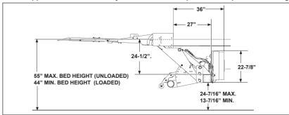
GPTLR-44 & 55 Lift Dimensions and Mounting Requirements
