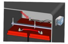
Step 5: Connect the positive wire with the in-line fuse to the positive post on the battery. Tighten battery nut.
