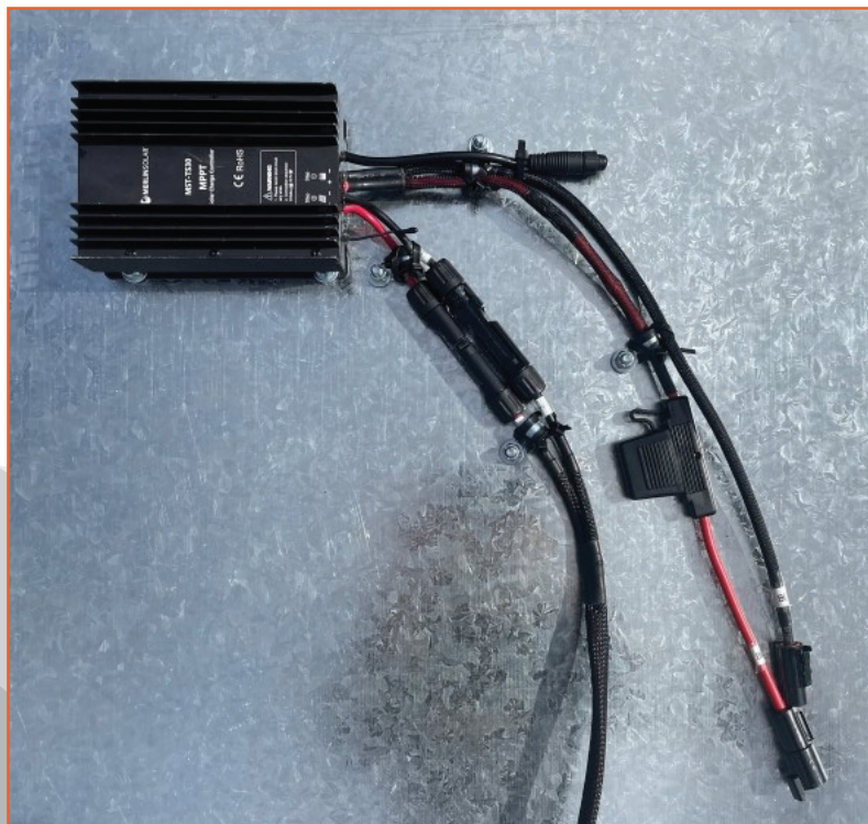
MERLIN® TS charge controller properly mounted and with strain relief.
