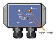
Figure 1: LEDs briefly turn green, toggle orange, then repeat
