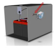
Note: The minimum hole size is 1.06 inches if there is not a pre-drilled hole in the battery box.
