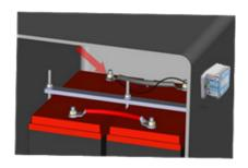
Step 5: Connect the positive wire with the in-line fuse to the positive post on the battery. Tighten battery nut.
