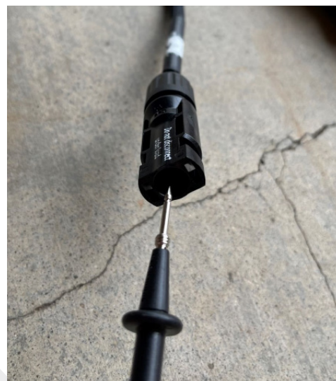
Insert BLACK (-) meter cable into PV- cable MC4 connector
