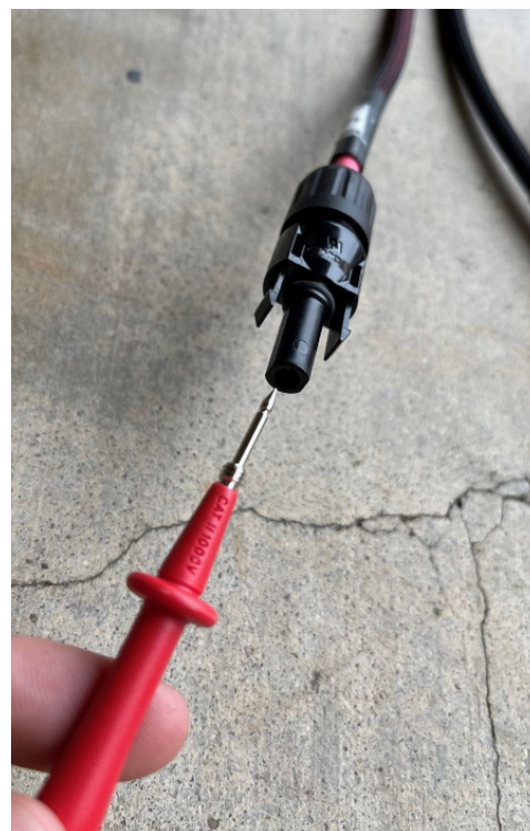
RED (+) meter cable into PV+ cable MC4 connector
