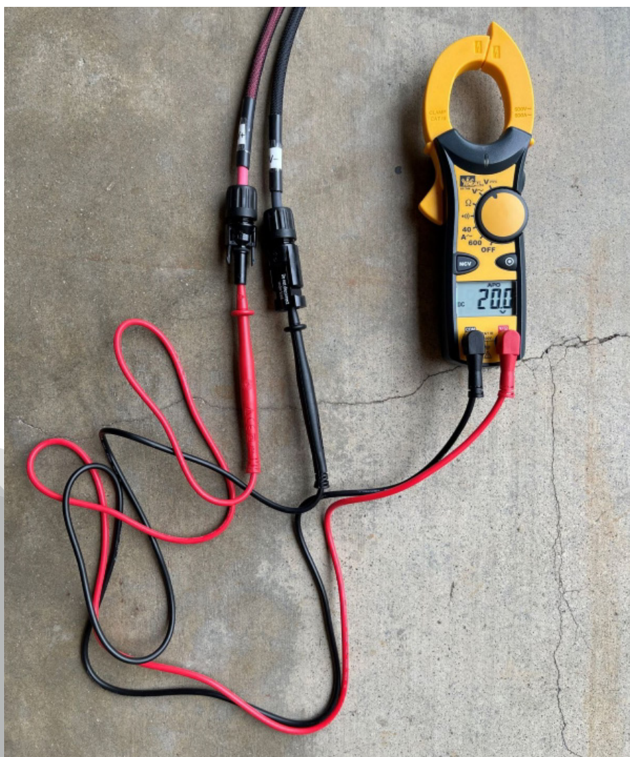
Multimeter displaying the connected PV's voltage
