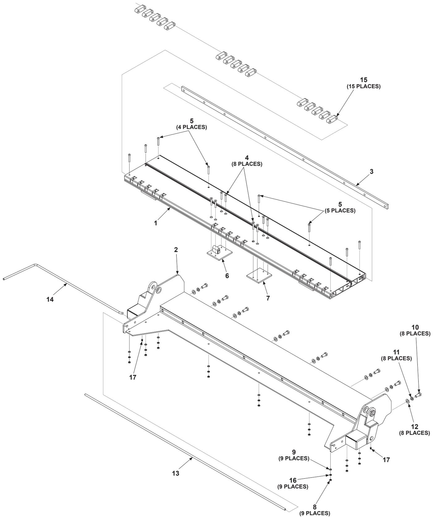
PLATFORM ASSEMBLY WITH 25" HEEL SINGLE TORSION BAR
