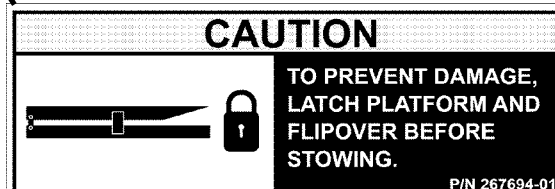
CAUTION DECAL (FLIPOVER EQUIPPED WITH LATCH ONLY) P/N 267694-01
