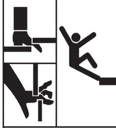
**Liftgate hazards can result in crushing or falling.**
