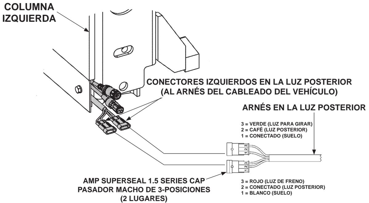
**CONECTAR EL ARNÉS EN LA LUZ POSTERIOR A LOS CONECTORES DE LA LUZ POSTERIOR (SE MUESTRA COLUMNA IZQUIERDA)**
